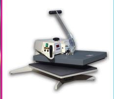
This swing head manual heat press is adapted for thicker items with the inclusion of a longer rear head post, that lifts the heat plate higher providing an additional 2.5cm clearance between the heat plate and table, which makes it possible to press onto thicker substrates.
