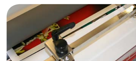
Automatic burst separating system separates sheets and delivers a clean datum edge from which to easily cut or guillotine
