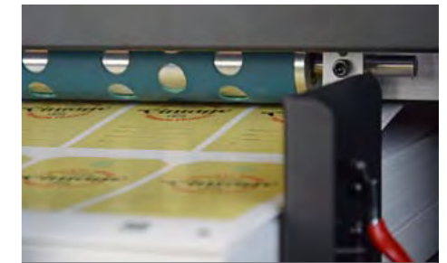
Continuous vacuum belt lifts and feeds sheets onto cutting bed ready for cutting
