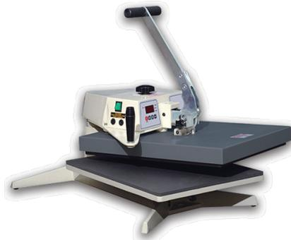
This swing head manual heat press is adapted for thicker items with the inclusion of a longer rear head post, that lifts the heat plate higher providing an additional 2.5cm clearance between the heat plate and table, which makes it possible to press onto thicker substrates.
