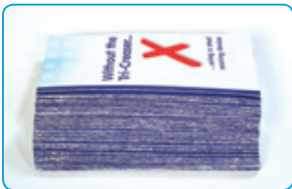
The type of damage a typical steel scoring device can do to the spines of cover stock material
