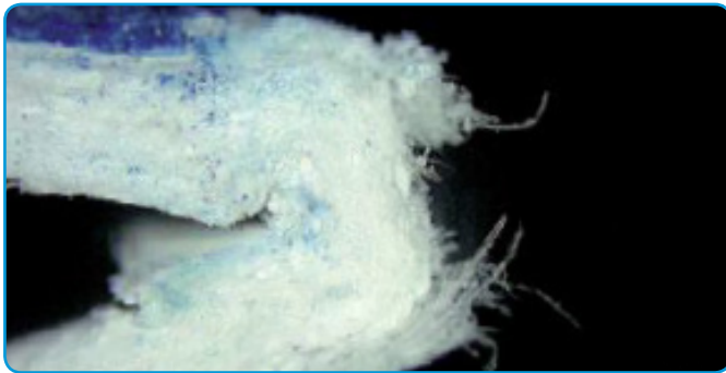
The pressure of steel causes damage to the outside of the fold
