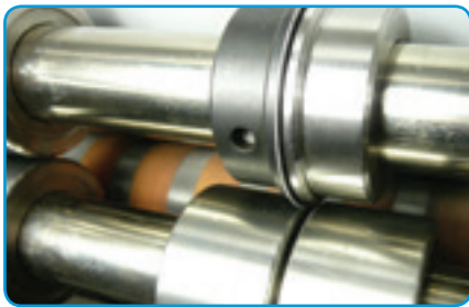
A typical steel scoring device supplied with all common types of folding machine
